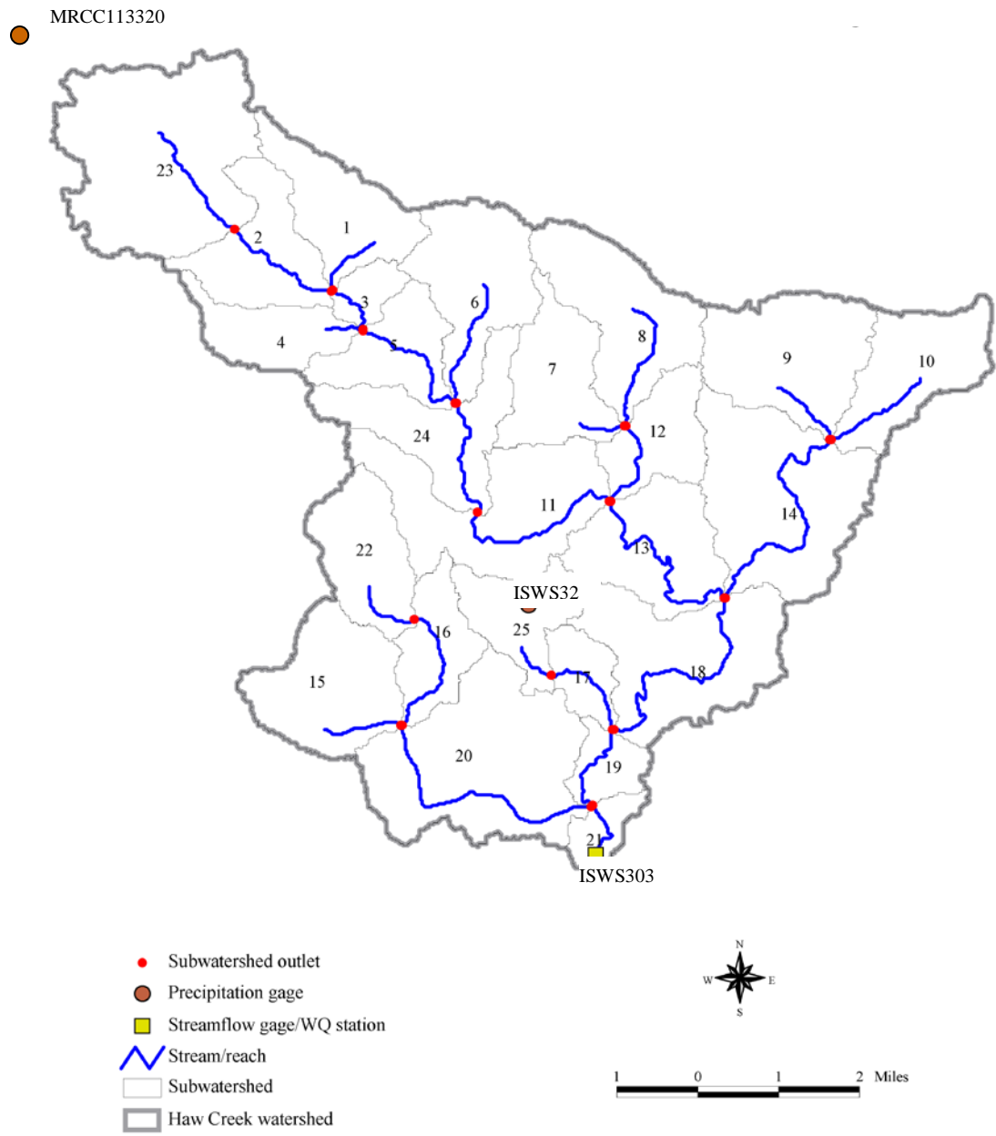
Figure 5-3. Schematic of the subwatershed and stream delineation, and precipitation gages used for the Haw Creek model
