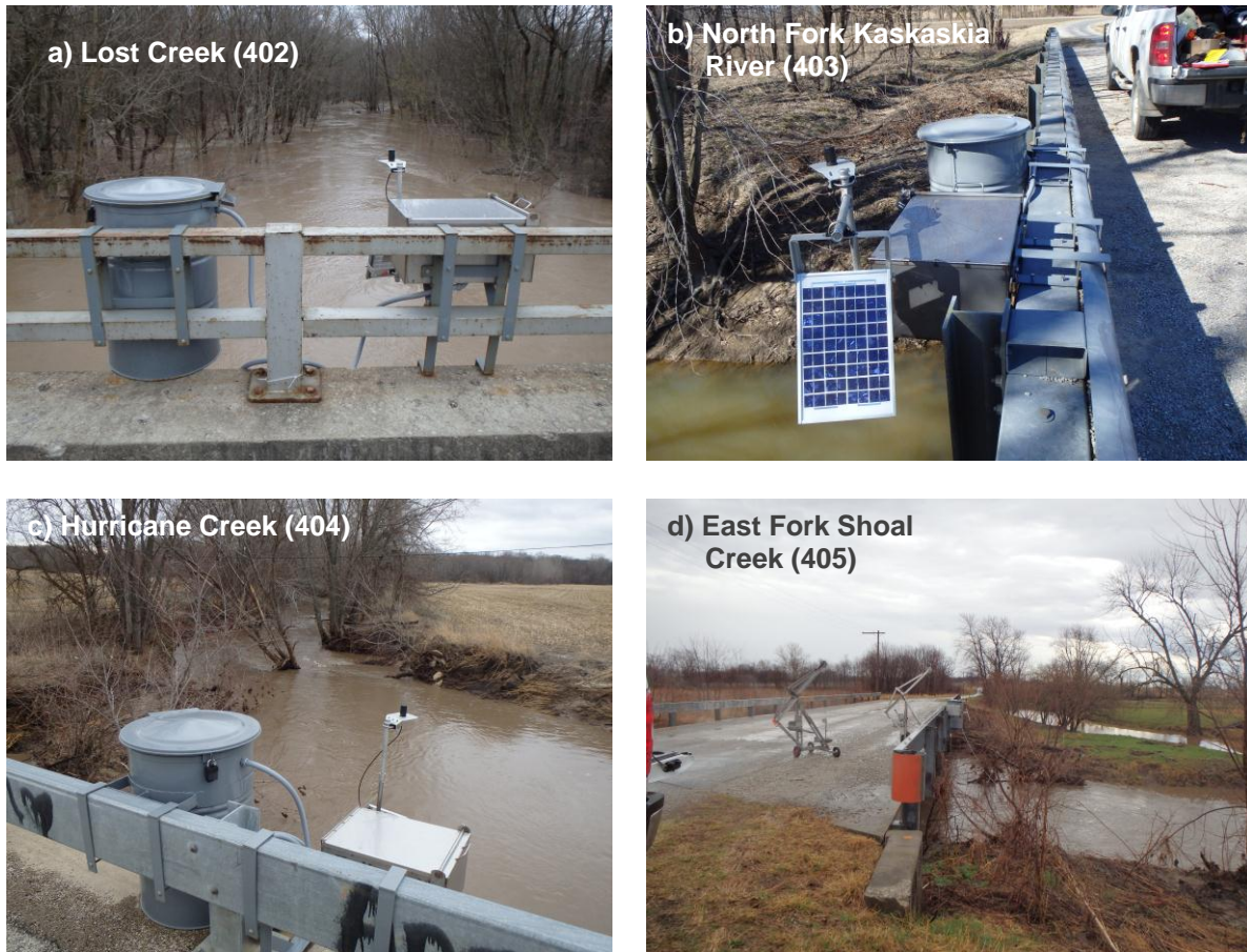
Figure 3-5. Streamgage monitoring stations in Kaskaskia River Basin: a) Lost Creek, b) North Fork Kaskaskia River, c) Hurricane Creek, and d) East Fork Shoal Creek
