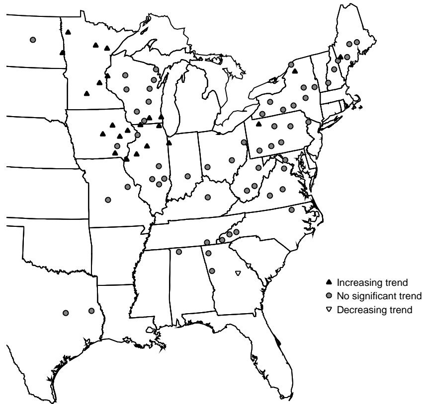
Figure 4-10. Locations of long-term streamflow gages (at least 89 years of record) showing statistically significant trends in mean annual flow in the eastern United States (from Knapp, 2005)
