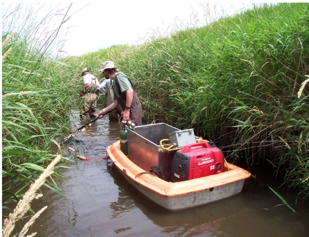
Figure 25. The two downstream treatment sites (EIE-18 and EIEM-01) are sampled using an electric seine powered by an AC generator, as shown here during a pre-restoration sampling event.
