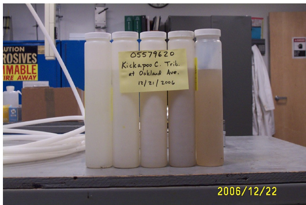
Figure 5. An example of suspended sediment samples collected for the Sediment Transport Study.
