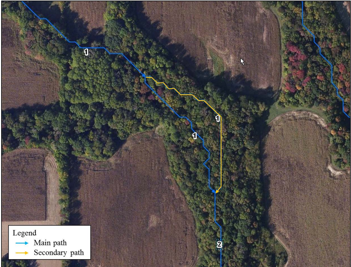
Figure AII.5. Stream order assignment error associated with secondary paths that increase the order of stream segments improperly. Stream order assignment issues occurred when a stream was classified as a secondary path (orange line) and was identified as an order 1 segment flowing independently into the main stream path (blue lines) instead of as a branch of the upstream reach during the GIS stream order assignment model. The GIS model was adjusted to correctly assign stream order.
