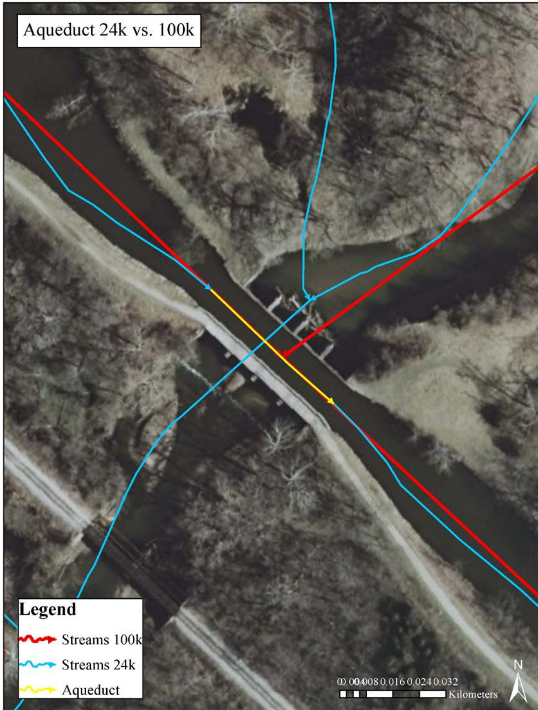
Figure AI.3. Aqueduct. We defined Aqueducts as portions of the digital stream network that flow over other stream segments in man-made structures. The 2005 stream network (red lines) merged the streams at their apparent confluence. However, there is no confluence on the landscape. Instead, the canal flows over the stream in an aqueduct (yellow line) while the other channel continues uninterrupted as reflected in the 2014 stream network (blue lines).
