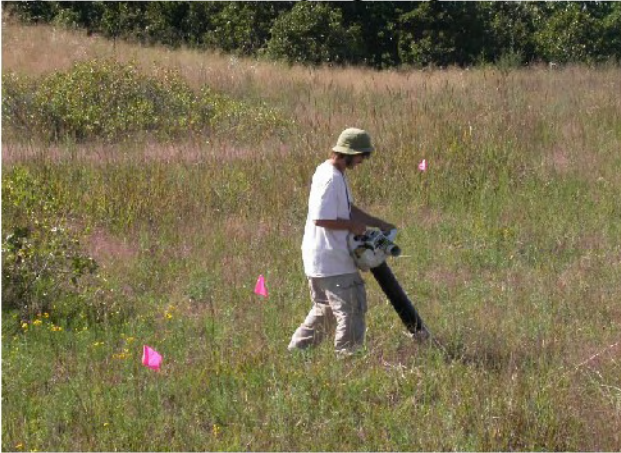
Figure 2. Vacuum sampling using a modified leafblower at Longbranch Prairie
