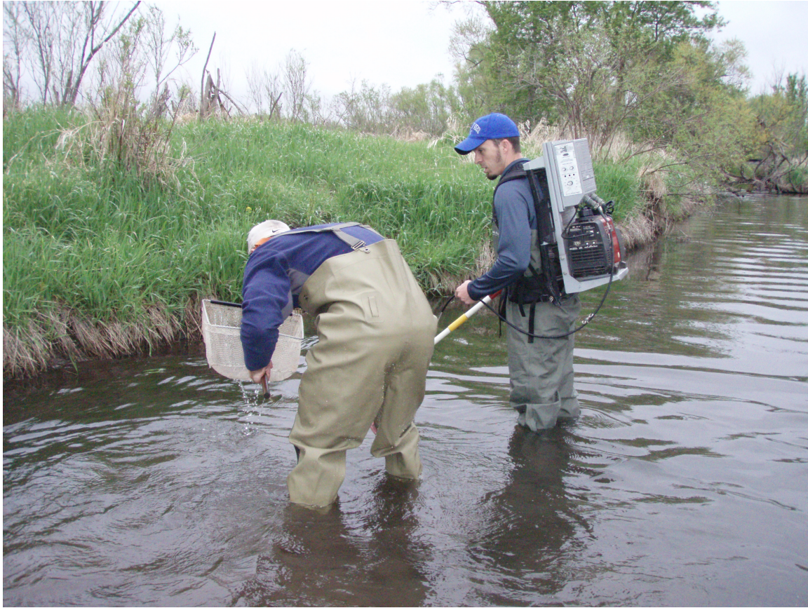
Figure 3. Sampling fishing using a Smith-Root Model 12 DC backpack electrofisher at Site 13 (IL: Winnebago County, East Fork Raccoon Creek, ~4.5 km NW Rockton, at Williams Tree Farm, which is where Clinostomus elongatus was found in 1998).
