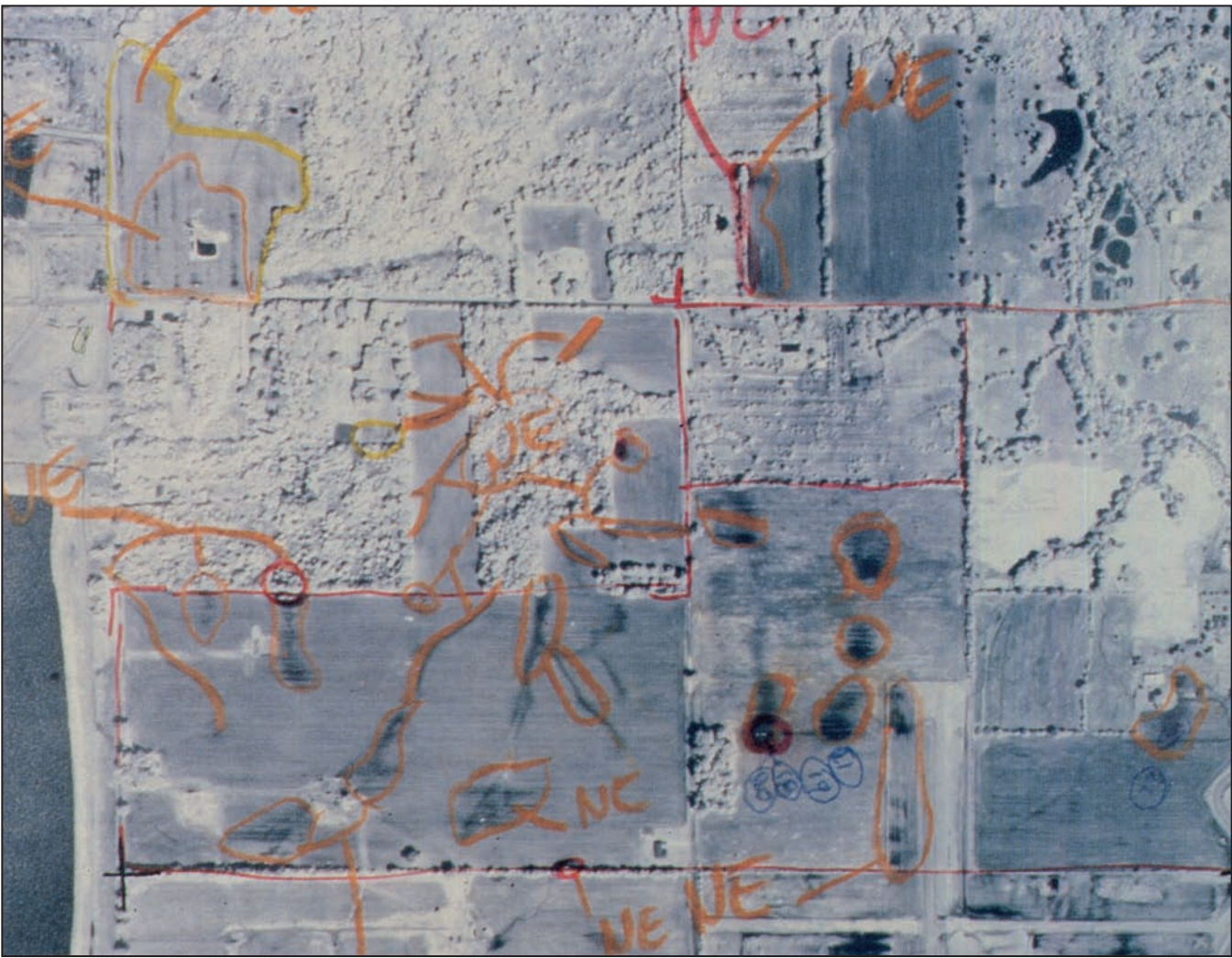
Figure 12 Aerial photos were used to locate subsided areas (circles) for study of the effects of unmitigated subsidence on corn yields.
