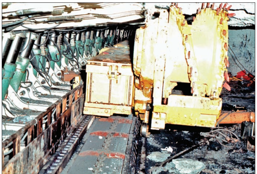
Figure 5 The longwall mining equipment photograph shows hydraulic shield supports (left) and cutting drum (right).
