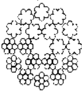
This rope has 18 strands of 7 wires each. It is an 18 x 7.
