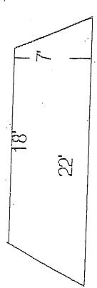
What is the area of this entry? The velocity is 90 fpm. What is the quantity of air?
