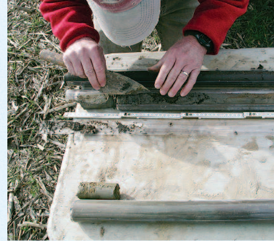
Using a geoprobe, drillers extracted cores of sediment to depths of more than 40 feet. Upon examination, the cores chronicle the history of the Illinois River.
