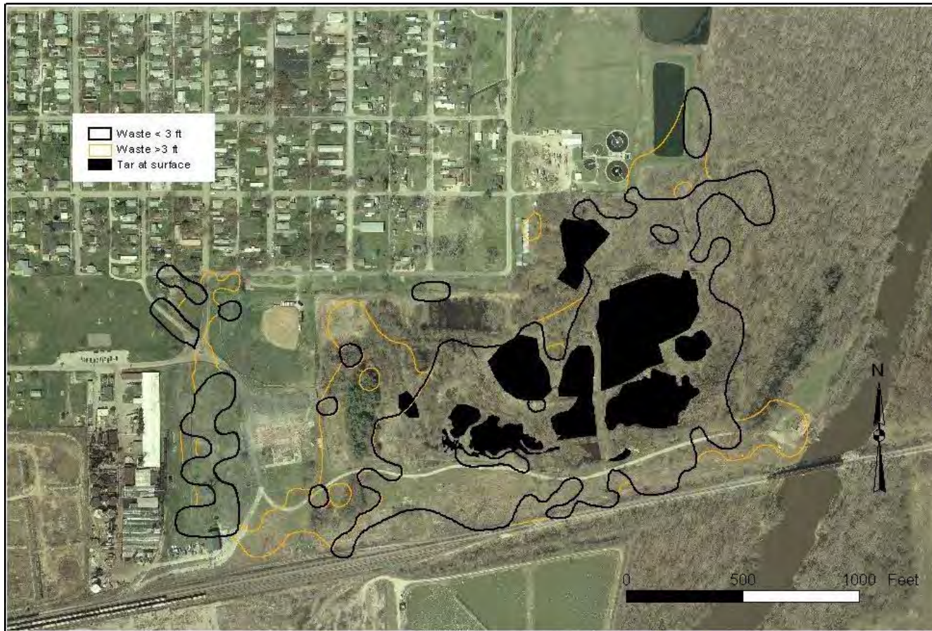
Figure 5.5. Areas with unvegetated tarry waste at the surface, tarry waste within the upper three feet of soils, and tarry waste below three feet. The State and Federal Trustees and Texaco incorporated this information into the injury quantification for Indian Acres.
