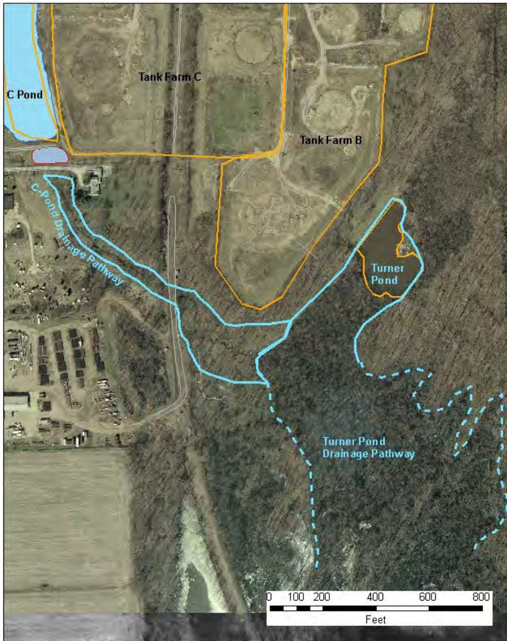
Figure 5.11. C-Pond drainage pathway, Turner Pond, and the Turner Pond drainage pathway, south of C-Pond and Tank Farms B and C. The dashed line outlines an area of lower elevation, based on a topographic survey (Trihydro, 2006). The estimated spatial extent of the Turner Pond drainage pathway for the purposes of the assessment is shown in Figure 5.1.
