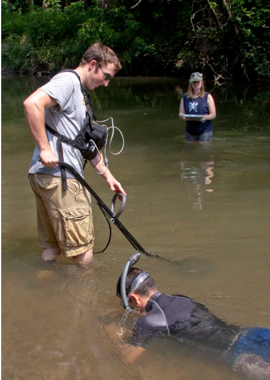
Figure 4. When surveying for PIT-tagged freshwater mussels, a person carrying a PIT tag receiver wand slowly sweeps the streambed while walking the stream in a systematic manner. Detected tags are stored in the PIT reader, and data are later downloaded into a database after the sampling period ends. At least one additional sampler snorkels (or uses view buckets) if conditions are favorable and visually examines the streambed for tagged mussels. If an animal is seen, a note is made whether it was alive or dead. Photo courtesy of Rob Kanter (U of I).
