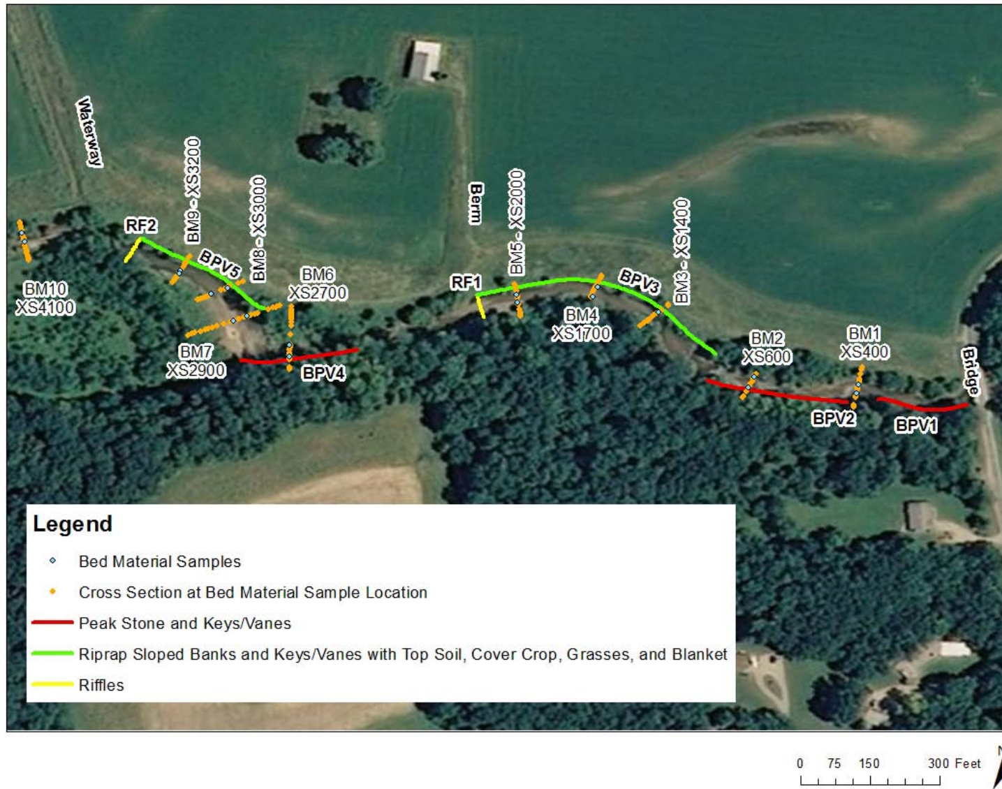
Figure 17. Location of bed material samples and surveyed cross sections at bed material locations.
