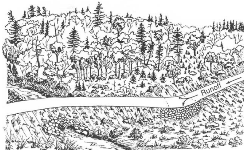
Figure 5-3. Place fill directly over a culvert higher than the road approach to prevent surface runoff from draining onto the crossing structure and into the stream.
