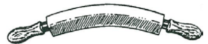
A quality fleshing knife has a sharp outer edge and a dull inner edge. The sharp edge is used to cut through and remove thick connective tissue from the back and neck. The dull edge can be used to flesh the sides and belly.
