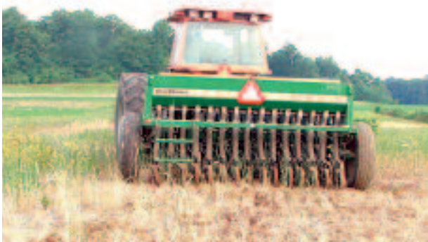
Herbicides must be used to kill fescue (top) before warm-season grasses can be successfully established using specialized grass drills (bottom)
